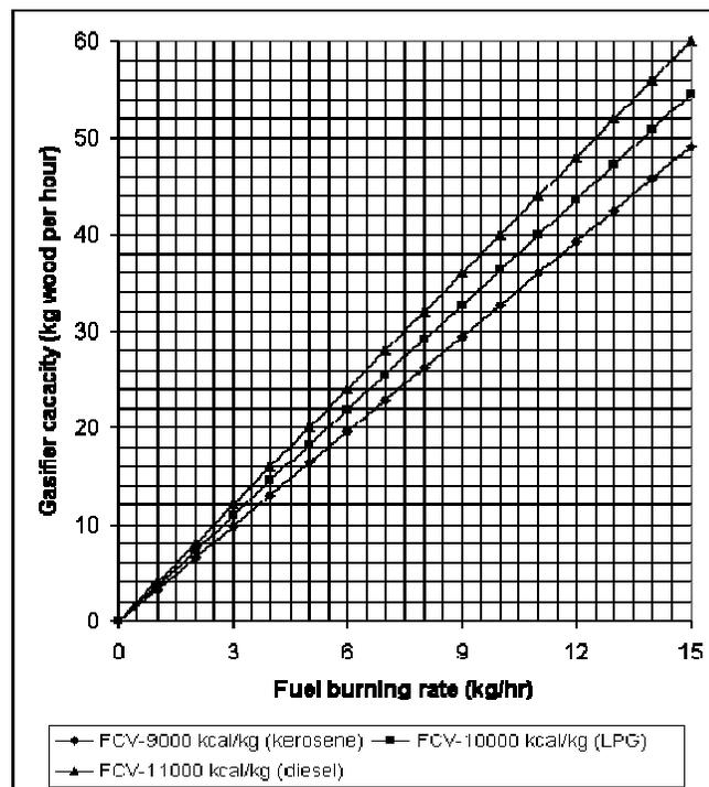
Figure 1.2 Gasifier sizing for replacing fossil fuels for thermal applications
