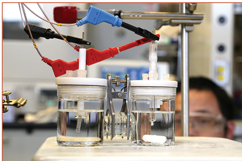
Electrolysing device that splits water into its component elements, oxygen and hydrogen (Credit: Marit Mitchell)
