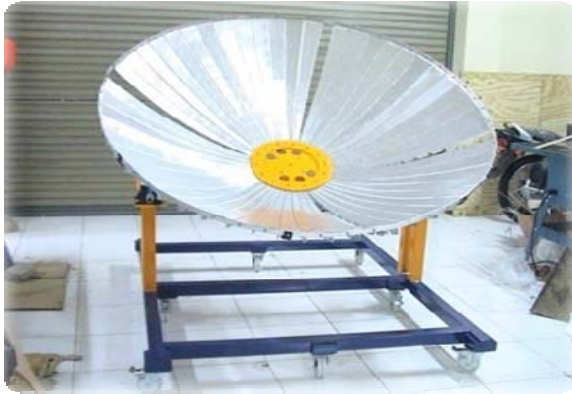
Figure 7.1. An example of Stove Solar Collector for Household Use. (Stove Diameter of 2 m) (Source : DEMR)
