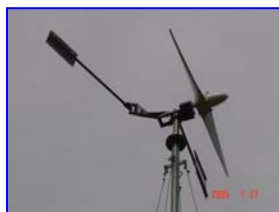
Figure 8.12 – Two-blade 100 W Wind Mill for Battery Charging
