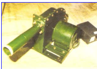
Figure 8.14 – Water Turbine 100 W (Source: - NERDC)
