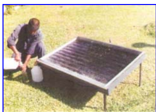
Figure 8.16 – Solar Distiller (Source: - NERDC)
