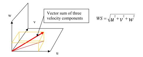
Figure 2.3 Three components of wind speed.
