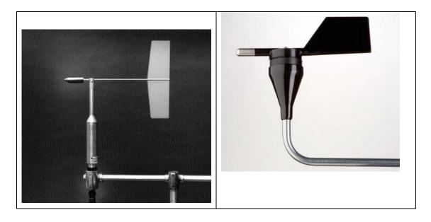
Figure 2.5 Typical Direction Vanes
