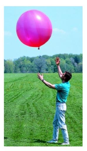
Figure 2.10 A Pilot Balloon being launched
