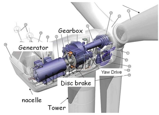
Figure 1.8 A typical modern Wind turbine
