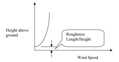
Most commonly used method for determining wind speeds at a heiht above ground refered to as the power law index method.
