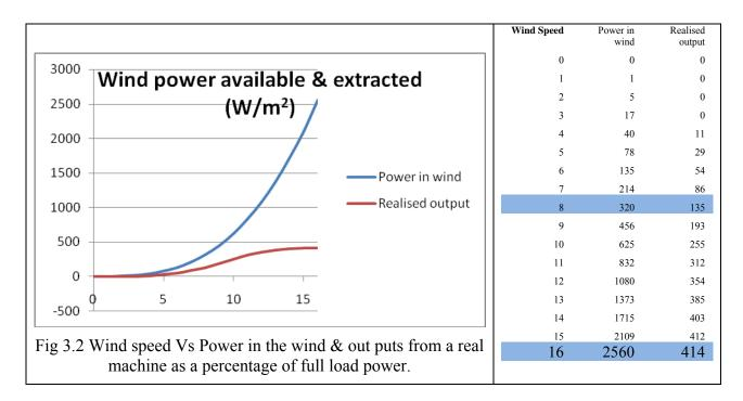
While designing a wind turbine it will be important to look at the frequency distribution a given location has and this is approximated using what are known as Weibull factors. Chapter 2 has dwelt on the distribution at some length. The excel sheet termed WEIBULL supplied with this material takes you through the computations and it should be possible to estimate approximate output energy at a given location.
