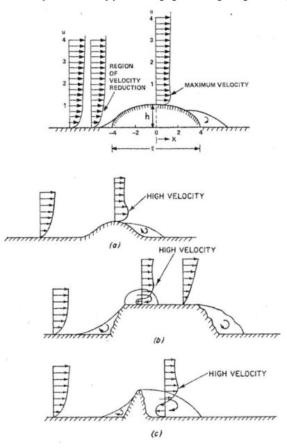
Figure 2.9 Velocity profiles changing with terrain changes (Adapted from C.J.Justus 1975)
