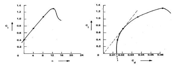
Figure 1.4 Dependence of Lift and drag coefficients on angle of attack (adopted from H.Lyson 1979)
