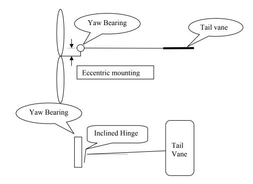
Figure 1.9 Passive Safety system for small windmills and wind battery chargers.
