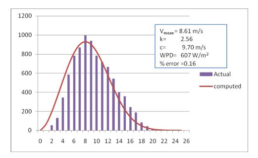
Figure 2.7 Actual & fitted frequency distribution. It is to be noted that though there seems to be a shift in the two distributions, the wind power density estimate has a small error.
