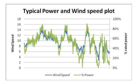
Figure 3.1 Typical time series plot of wind speeds and corresponding power It may be seen that the power falls rather rapidly with lower speeds and ramps up and down far more rapidly as the wind speeds increases or decreases. This can be understood by the following:
