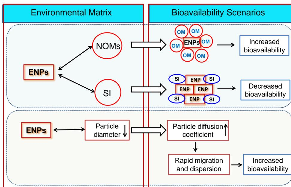
**Figure 2: Availability of engineered nanoparticles after interaction with different environmental matrixes**
