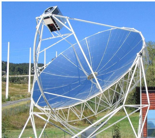
**Figure 15:** Dish Stirling (Source: intersol.se)
