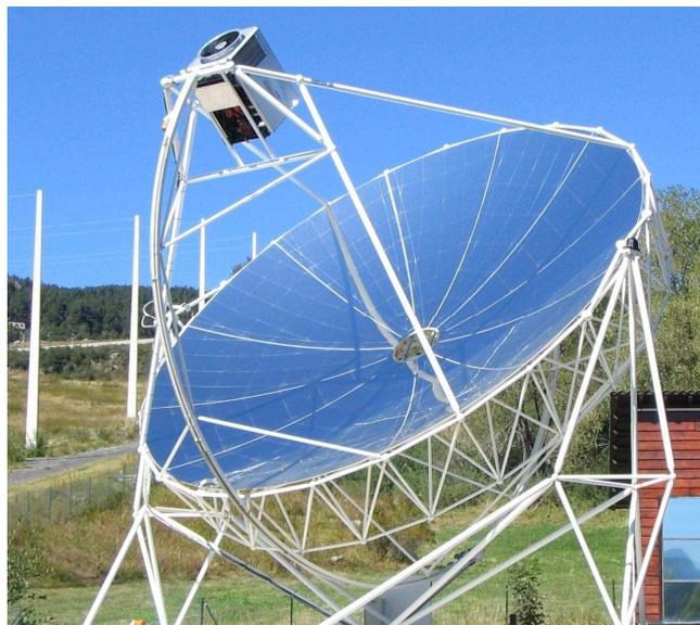
**Figure 15:** Dish Stirling (Source: intersol.se)
