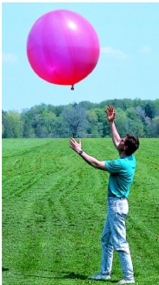
Figure 2.10 A Pilot Balloon being launched
