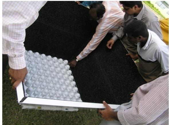
SODAR being set up for measurements
