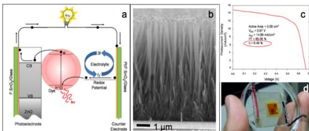
**Figure 10: Dye-sensitized solar cells (DSSC). The electron transport scheme is shown in (a). The ZnO nanorods are shown in (b). A sample current-voltage curve is shown in (c). (d) depicts a DSSC.**
