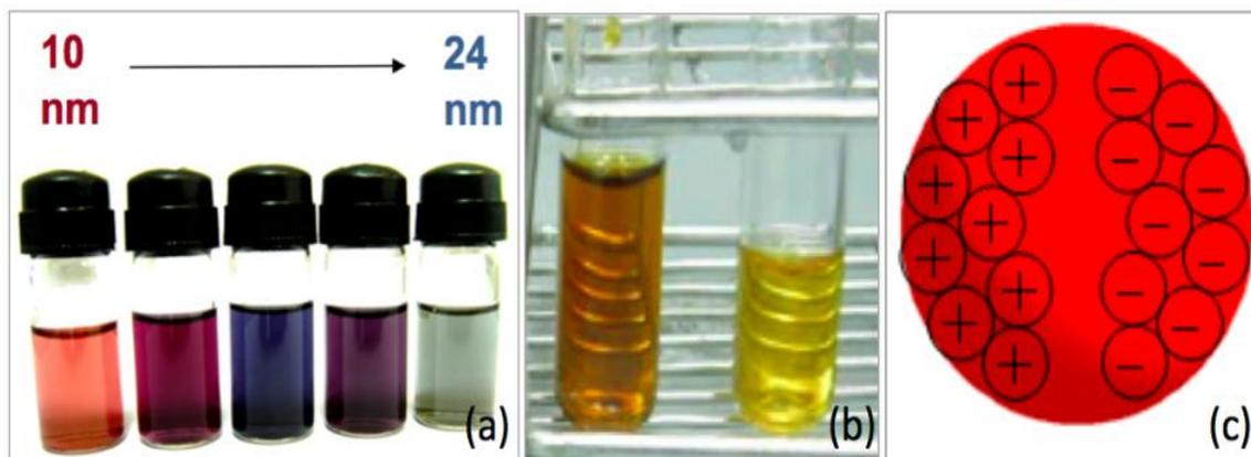
**Figure 15: The various colors of gold nanoparticles are shown as a function of size.** (Image courtesy: Center of Excellence in Nanotechnology, Asian Institute of Technology)
