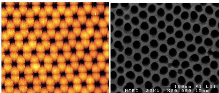
**Figure 19: Porous and honeycomb-like structure of alumina membranes. On the left, an atomic force microscope (AFM) image of membrane with 80 nm pore diameter and on the right, a scanning electron microscope (SEM) image of a membrane with 100 nm diameter pores are depicted.** (Image courtesy: Center of Excellence in Nanotechnology, Asian Institute of Technology)
