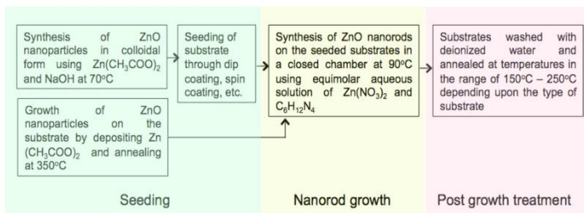
**Figure 8: Synthesis of ZnO is straightforward and cost effective– it all depends on chemistry from the bottom-up** (Image courtesy: Center of Excellence in Nanotechnology, Asian Institute of Technology)
