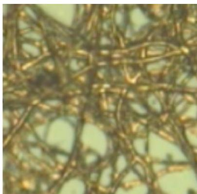
**Figure 18: Gold nanotubes made from templating effect of hyphae of *Aspergillus niger*, the common mold**
