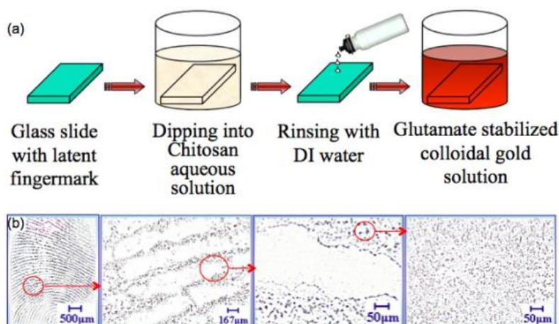
**Figure 16: A new fingerprint detection method based on gold colloids** (Image courtesy: Center of Excellence in Nanotechnology, Asian Institute of Technology)
