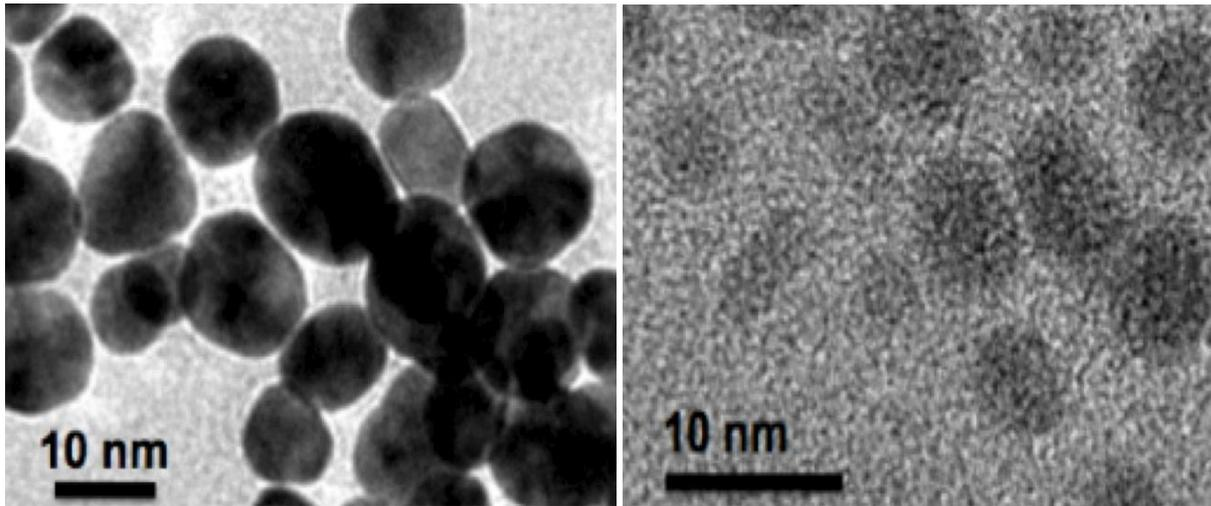
**Figure 6: Transmission electron micrographs (TEM) of Au and ZnS nanoparticles electrostatically stabilized through steric hindrance by coating with a biopolymer called chitosan** (Image courtesy : Center of Excellence in Nanotechnology, Asian Institute of Technology)
