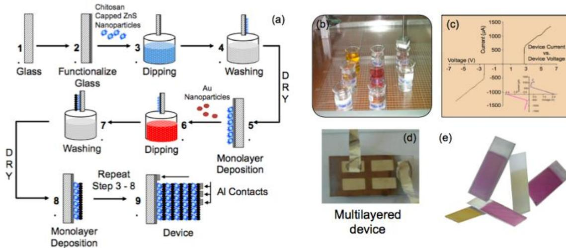
**Figure 14: A Layer-by-Layer (LBL) scheme of structure**
