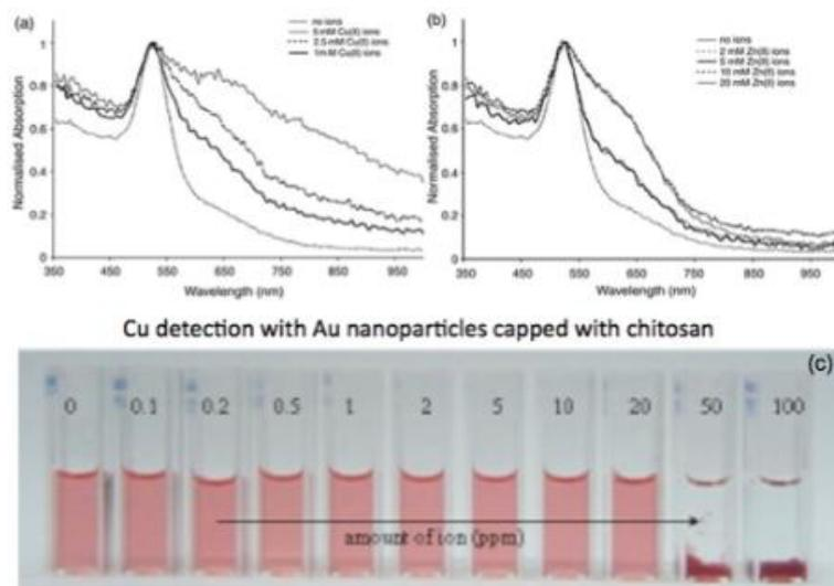
**Figure 17: A comparison of the optical absorption spectra of the colloidal gold nanoparticle suspension before and after exposure to metal ions** (Image courtesy: Center of Excellence in Nanotechnology, Asian Institute of Technology)
