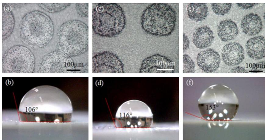
**Figure 13: Superhydrophobic surface created by use of ZnO nanorods and other structures. The water contact angle can be affected by control of the spacing of the microbumps and the height of the ZnO rods.**
