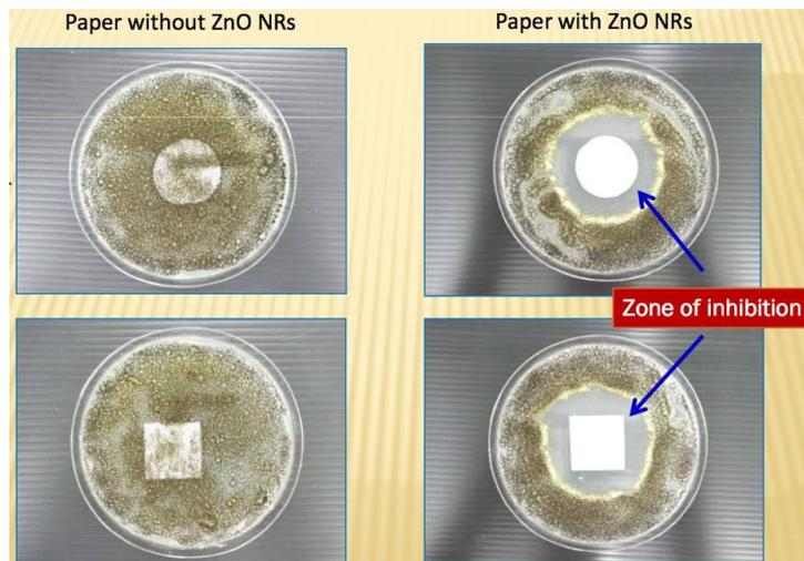
**Figure 11: ZnO-treated paper showing antimicrobial properties against the common mold *Aspergillus niger***
