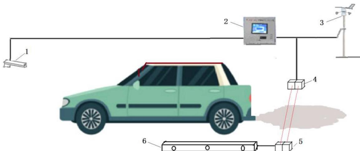
**Figure 7.10:** Schematic of vehicle emission remote sensing system. 1. License plate camera; 2. main control computer; 3. weather station; 4. light source and detector; 5. reflector; 6. Speedometer (Ren X. et al., 2022)
