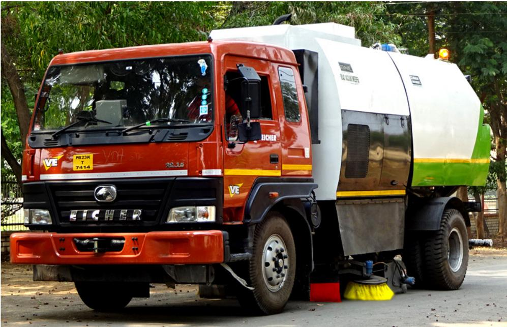
**Figure 7.6:** Road sweeping truck with vacuum sucker for road dust
