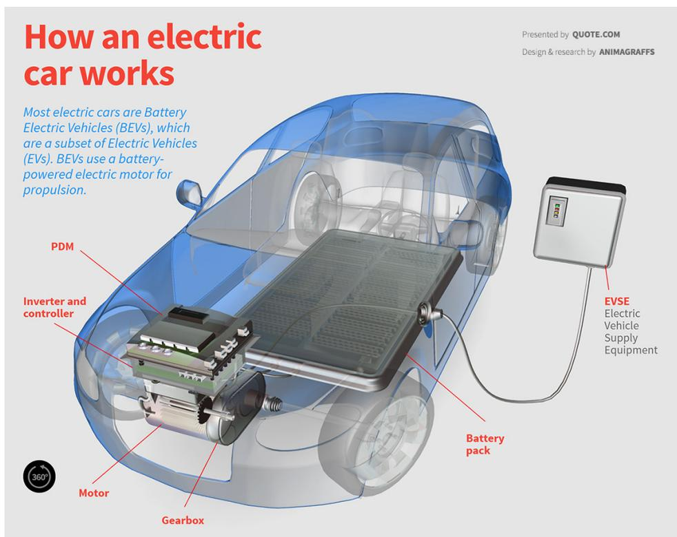
Figure 7.5: Battery electric vehicles (BEVs) [source: Animagraffs]
