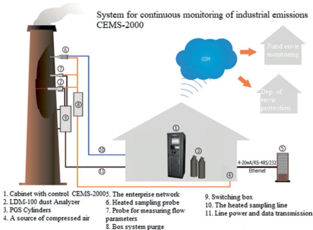
**Figure 7.11:** Component of CEMs (Tsymbalov, S.D., et. al (2022))
