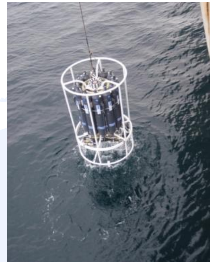
SBE ECO-55 carousel with 4 liter Niskin bottles
