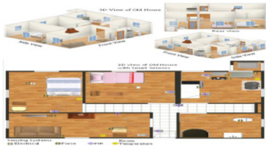
Figure 7b: Placement of sensors in an old home to convert it to a technology assisted home
