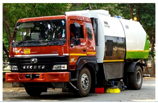
Figure 7.6: Road sweeping truck with vacuum sucker for road dust
