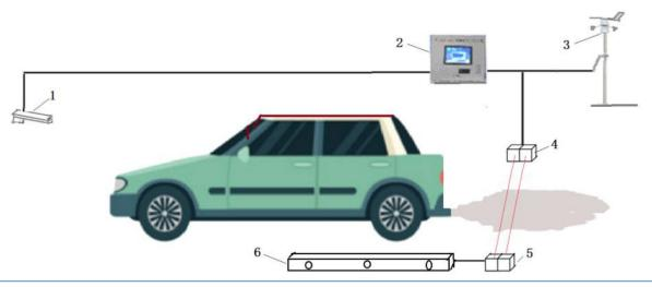
**Figure 7.10:** Schematic of vehicle emission remote sensing system. 1. License plate camera; 2. main control computer; 3. weather station; 4. light source and detector; 5. reflector; 6. Speedometer (Ren X. et al., 2022)
