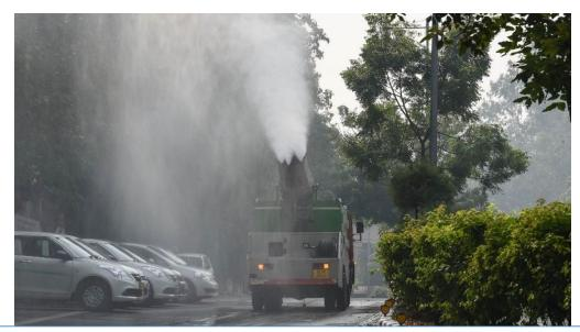
Figure 7.7: Truck mounted anti-smog gun to spray water droplets to curb air pollution
