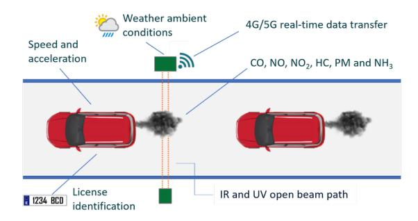
Figure 7.9: Remote sensing for vehicle inspection (OPUS, 2023)
