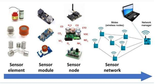
Figure 7.1: Typical Low-Cost Sensors for Pollutants Monitoring [Penza, M. (2020)]
