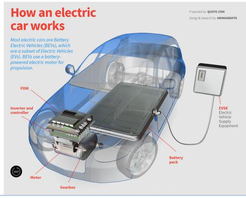
Figure 7.5: Battery electric vehicles (BEVs) [source: Animagraffs]
