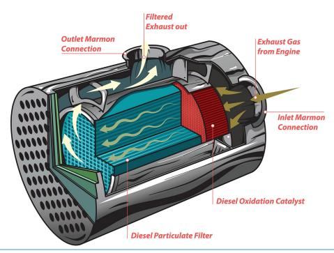
Figure 7.3: Diesel Particulate Filter for diesel vehicle emission control (DPF)
