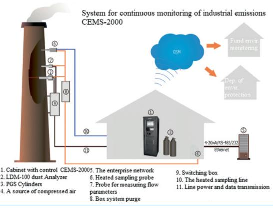
Figure 7.11: Component of CEMs (Tsymbalov, S.D., et. al (2022))
